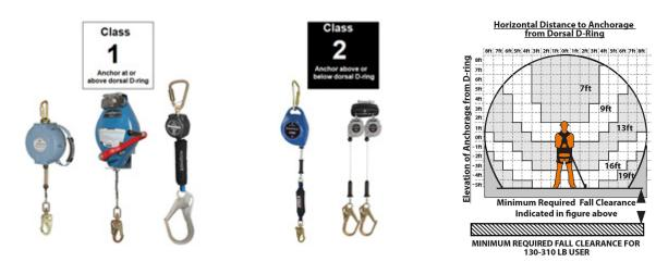
In addition to the Class 1 and Class 2 standard labels, all Class 2 SRLs must include a full fall clearance table or diagram on the physical product, not just in the user instruction manual. This places critical clearance information directly on the product, where it is most easily accessible by the end user or Competent Person.
